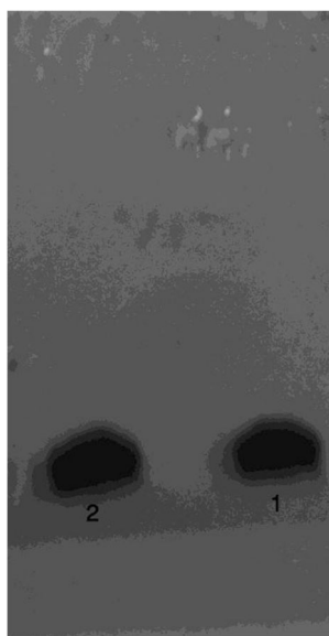
Fig. 8. SDS-PAGE result for intact insulin (1) and releases of insulin from SMGel after 35 days (2)
